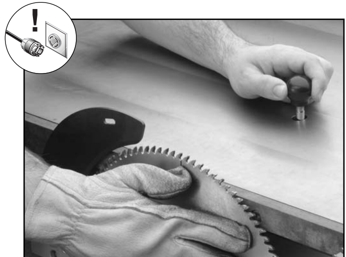
Figure 81. Locking main blade with the lock tool.
